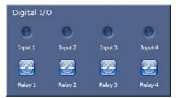
The alarm icons **Input 1** to **Input 4** are for information purposes and indicate the status of an alarm input: When an alarm is triggered, the corresponding icon lights up blue. The unit's configuration determines whether the alarm is displayed, as well as additional details (see *Section 5.15 Advanced Mode: LIVEPAGE Functions, page 43*).
